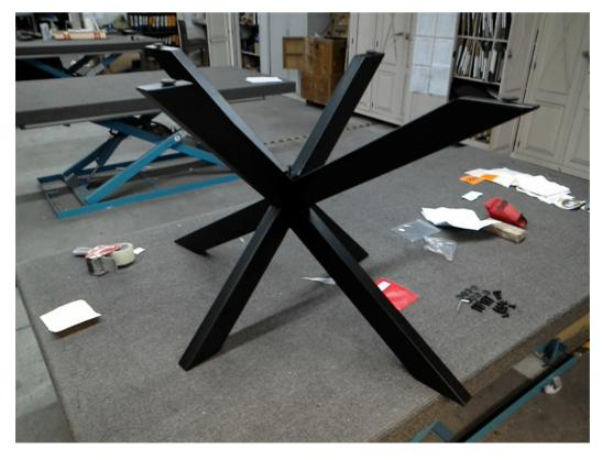
assembled powdercoated central leg, after leg assembly it can be connected to top. After that all screws/bolts can be tightened,
