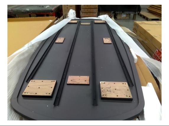
Assembly blocks for legs and anti bending irons to prevent table from bending.
