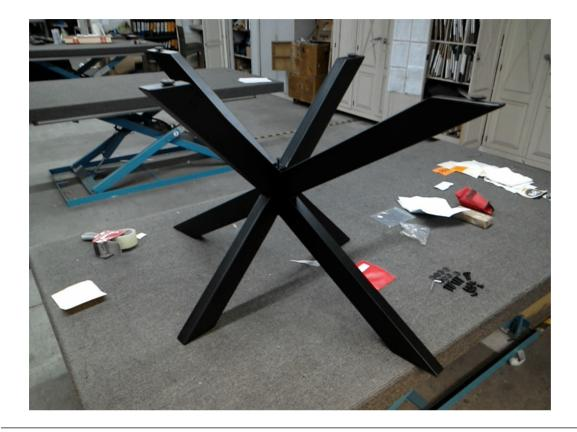
assembled powdercoated central leg, after leg assembly it can be connected to top. After that all screws/bolts can be tightened,
