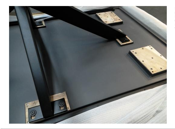
leg assembly, make sure top plates are mounted correctly, otherwise one will be not able to assemble the table.
