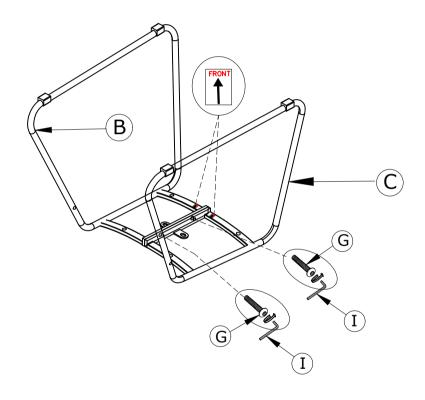
2 Step 2: Insert horizontal bar with the small hole (at center) pointed up. !careful not to scratch the frame!
