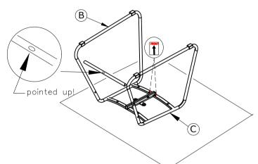
3 Step 3: fasten the horizontal bar for 100%.
