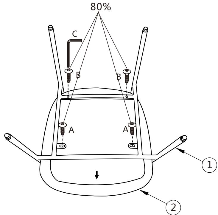
② MAKE SURE THE GAP OF TWO SIDES ARE EQUALIZED
